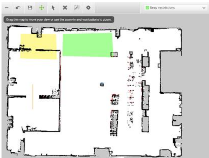
Figure 8.4. Narrow doorways can be marked with a Sound and light zone (marked with yellow) to warn people that it is coming through. A Critical zone (orange) can be placed on the narrow doorway to force the global planner to make a path through the corridor.
